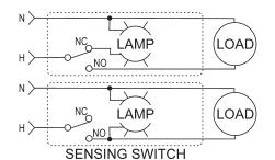
**OFF** indication with HOT and NEUTRAL: lamp glows when load is **OFF**.
