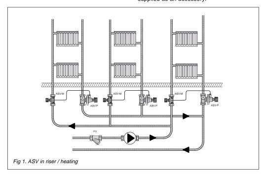
ASV valves are to be used in radiator heating systems to control the differential pressure in risers. To limit the flow for every radiator, the thermostatic radiator valve with pre-setting facilities (feature) is used together with a constant pressure provided by the ASV, thus providing balanced heat distribution. Alternatively the flow in the riser can be limited by using setting function of the ASV-I.
