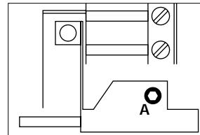
**15** Turn screw **A** with an Allen key until the switch changes over when the valve is open:
