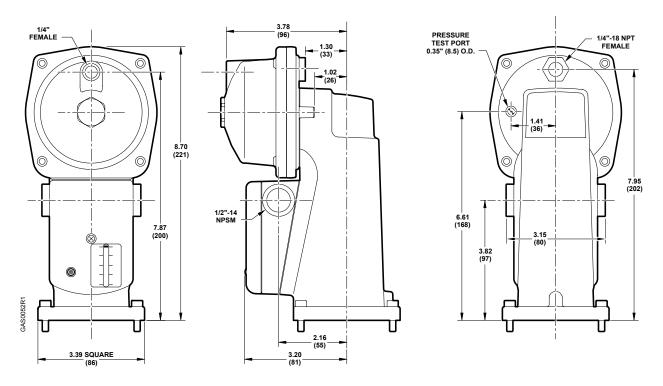
Figure 3. SKP25...U.. Dimensions in Inches, Millimeters in Parentheses.
