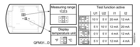
The setting elements are located inside the cover. A setting element is consisting of 6 pins and a shorting plug. It is used for selecting the required temperature measuring range and for activating the test function. Types with LCD display have a second setting element with 4 pins and a shorting plug.
