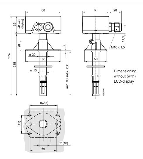
Drilling template with (without) mounting flange
