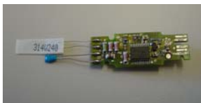
Figure 3. Q-Series Relative Humidity Removable Sensing Element (Replacement Part AQF3050).
