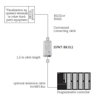
The connection to the MPI bus can be extended with an additional cable. For that purpose, Systeme Helmholz GmbH offers the following products:
