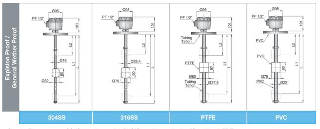
■ Special Float: 2" - 316SS (Ø52 x H60mm) & PVC(Ø50x H80mm) with JIS 10K 50A FF Flange
