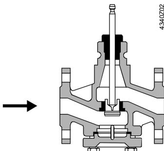
For all nominal sizes, a guided slot plug is used that is directly connected to the valve stem.
