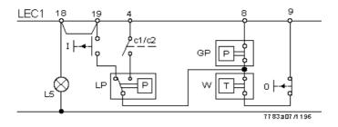
Connection examples for burner operation are given in data sheet 7761 for the control unit LEC1...
