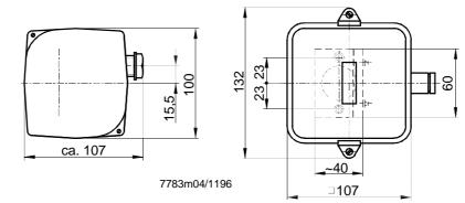
UV detector QRA50... (with mounting coupling) for mounting onto a viewing tube UV detector QRA51... for burner mounting
