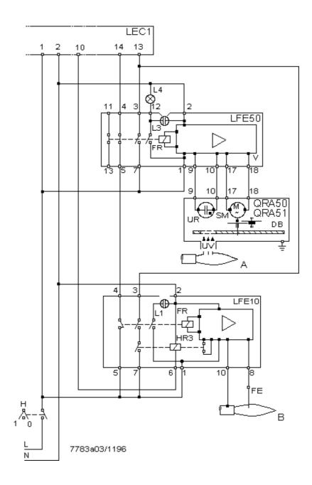
Supervision of the pilot burner (B) using an ionization detector electrode «FE» and a flame safeguard LFE10 (up to completion of the 2nd safety time).
