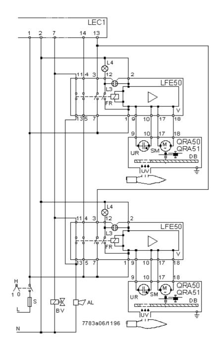
This circuit is used when burner operation must be maintained even in the event of a fault in the flame supervision circuit. With failure of a flame safeguard or a UV cell - signalled by a horn or similar - self-checking supervision is maintained by the second system. This allows the fault to be corrected without having to shut down the burner. Flame supervision of the main flame (A) of an interruptedpilot burner with DETACTOGYR
