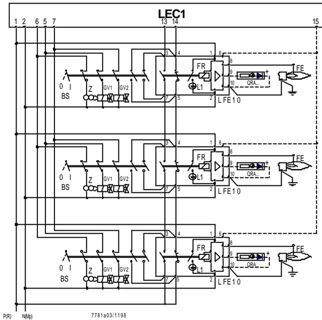
Like with dual-supervision, the control contacts of the flame relays of all flame safeguards must be connected in series.
