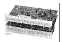
Microprocessor-based gas burner controls providing all control functions required by modern gas-fired heating boilers in intermittent operation with automatic ignition LGM11.34... have been designed for use in small gas heaters (wallmounting or floor-standing) with modulating premix burners, offering high efficiencies and extremely low emission levels.
