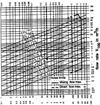
Recommended selection in  $\Delta Pv100$  =0.3Bar 1m<sup>3</sup>/h = 0.278kg/s water at 20°C
