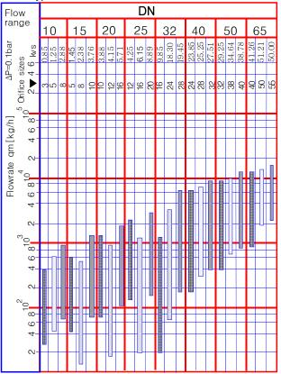
Recommended selection in  $\Delta P_{v100}$  =0.3Bar 1m3/h=0.278kg/s water at 20  $^{\circ}$ C
