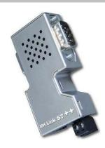
The *IBHLink* **S7** is an Ethernet-converter within a 15-pin Sub-D-housing for a connection via a switch, a hub or even directly to a PC with a common network adaptor. The protocol used is the standard TCP/IP protocol. In this way, the user can benefit from all the advantages of Ethernet, such as remote maintenance via a standard router or VPN-connections (Virtual Private Network). Likewise, a direct connection to the Internet is possible.
