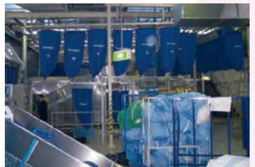
Section of the monorail bag system
