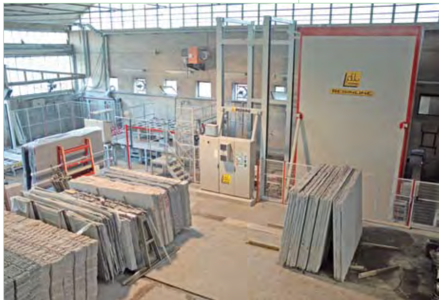
View of a Pedrini Marble oven machine installed at manufacturing site
